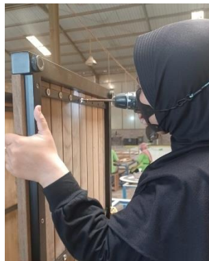
Gambar 3. Pemasangan coffee table menggunakan mesin bor tangan Figure 3. Installation of coffee table using hand drilling machine
