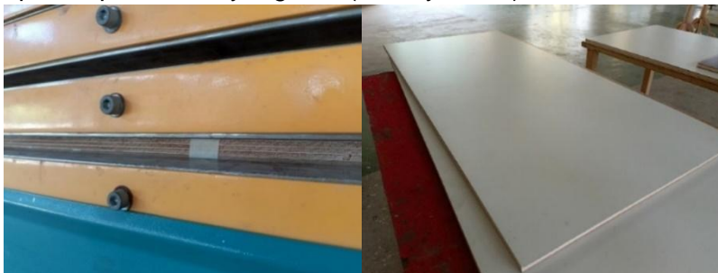
Gambar 4. Proses kempa panas dan hasil pengaplikasian HPL Figure 4. Hot felting process and HPL application results
