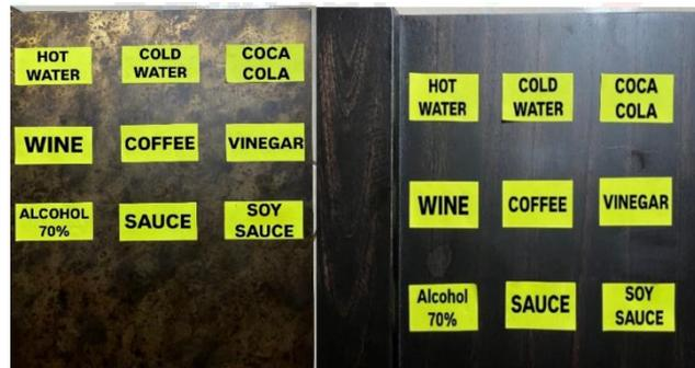
**Gambar 2. Hasil Uji ASTM D-1654 Pada Panel Finishing**
