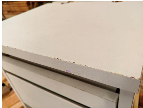
Gambar 11. Kendala bagian PVC sheet pecah Figure 11. Obstacle of PVC Sheet Part Breaking
