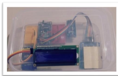
Gambar 2. Bentuk alat pengukur kecepatan aliran air Figure 2. The form of a water flow velocity measuring device.
