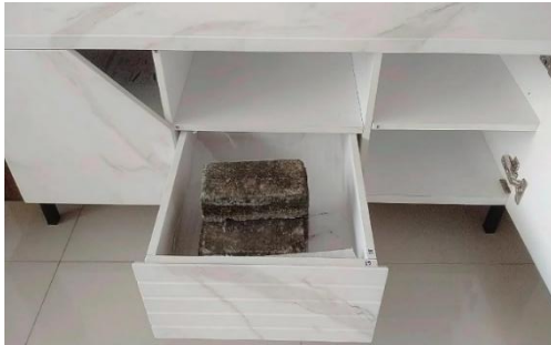
Gambar 7. Uji Beban Laci Tv Stand Figure 7. Tv Stand Drawer Load Test Sumber: Dokumentasi Pribadi, 2025
