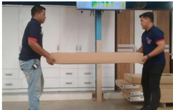
Gambar 11. Proses Drop Test Duspack Produk TV Stand Minimalis Modern Future 11. Drop Test Process for Duspack of Modern Minimalist TV Stand Products Sumber: Dokumentasi Pribadi, 2025
