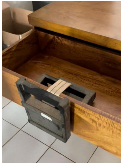
Gambar 7. Pengaplikasian beban uji 27,5 kg Figure 7. Application of 27,5 kg load test
