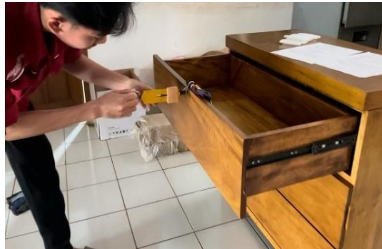
Gambar 5. Uji Gaya Horizontal Napali Drawer Dresser Figure 5. Horizontal Force Test of Napali Drawer Dresser
