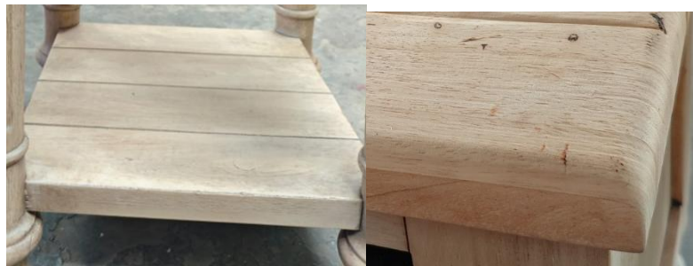
Gambar 10 Pembentukan Garis Alur dan Radius Figure 10 Formation of Contour Line and Radius
