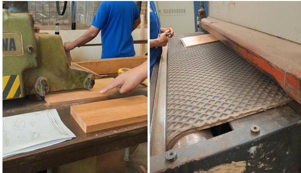
Gambar 5 Proses Pemotongan dan Penghalusan Kayu Figure 5 Process of Cutting and Smoothing Wood
